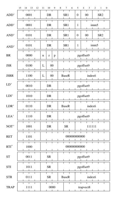
Figure A.1: Formats of the 16 LC-2 instructions. NOTE: + indicates instructions that modify condition codes; \* indicates that meaning and use of RTI is beyond the scope of this book.
