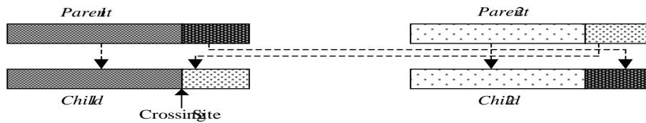
Figure 48: Schematic of simple crossover
